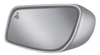
Figure 2: Ford blind spot detection visual indication (Source: Ford)
